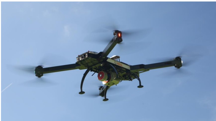
Figure 16: RiCOPTER developed by Riegl with laser-scanning equipment (Riegl, "UAS/UAV Gallery," http://www.riegl.com/nc/products/unmanned-scanning/gallery/ )
