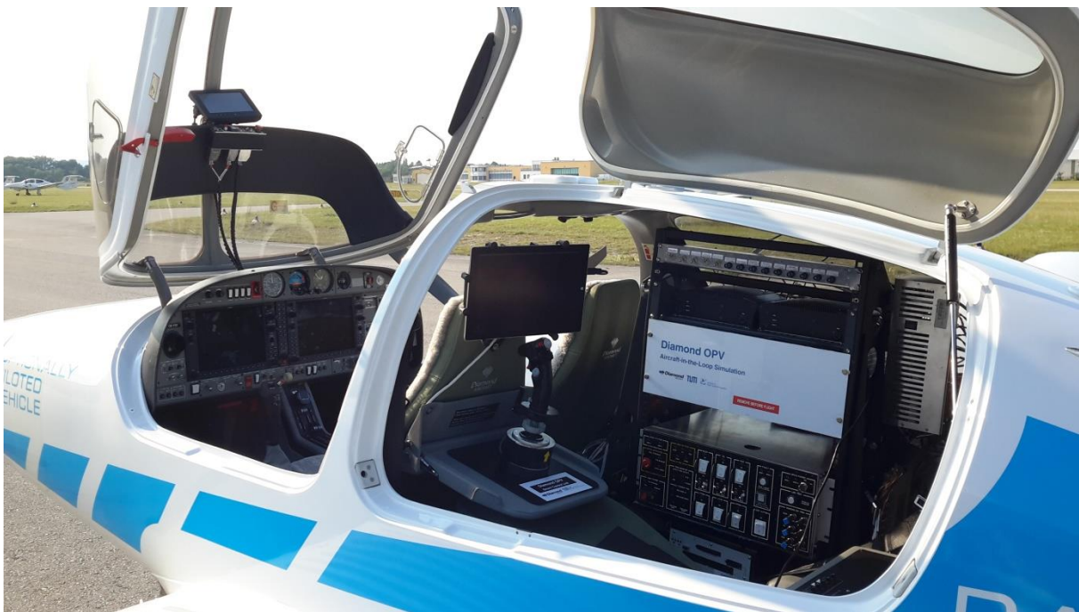
Figure 15: Interior of a DA42 MPP with visible experimental OPV electronics (AbsInt, "User story: TU Munich, Institute of Flight System Dynamics," https://www.absint.com/tum_fsd.htm )
