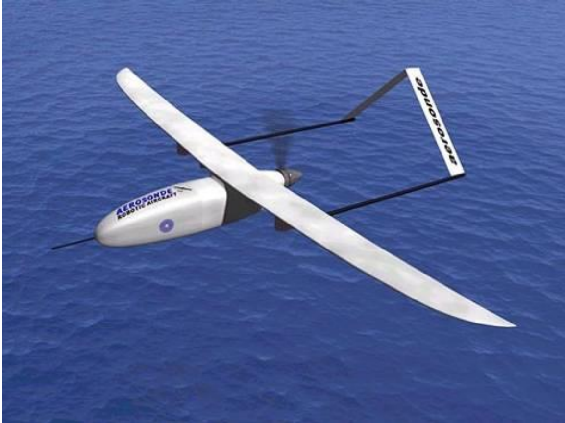
Figure 13: The Aerosonde Mark I "Laima" used for the first Atlantic crossing with a UAS (Flight Global, "First Atlantic crossing by an Unmanned Aircraft," http://www.barnardmicrosystems.com/UAV/milestones/atlantic_crossing_1.html )
