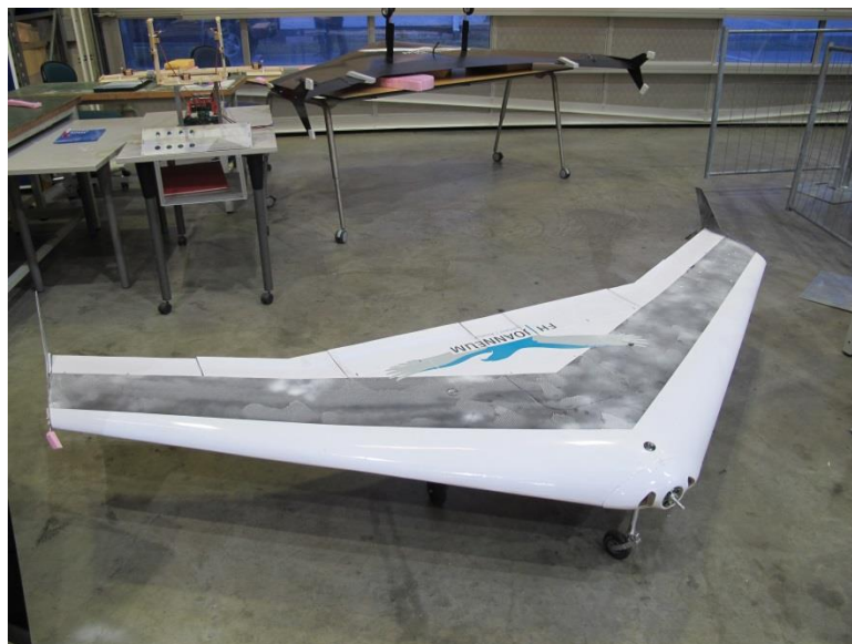
Figure 18: JXP-V fixed-wing UAS developed by the Joanneum University of Applied Sciences
