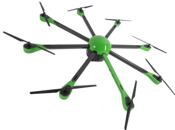
Figure 17: twinMAX developed by TWINS for the transportation of heavy payloads (Twins, "Flugplattformen," http://www.twins.co.at/de_DE/produkte/flugplattformen/ )
