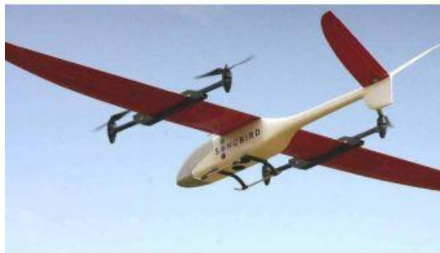
Figure 5: Hybrid-UAS with rotor blades in the horizontal pose (GIM International, "Hybrid UAS/UAV: Fixed Wing and Chopper in one Aircraft," https://www.gim-international.com/content/article/hybrid-uas )
